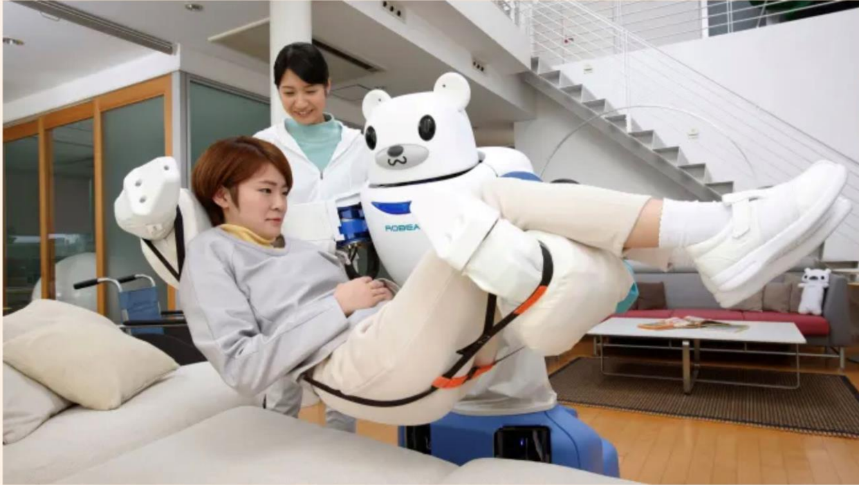
Grin and bear it: the Robear robot can lift elderly people or hospital patients off their bed into a wheelchair
